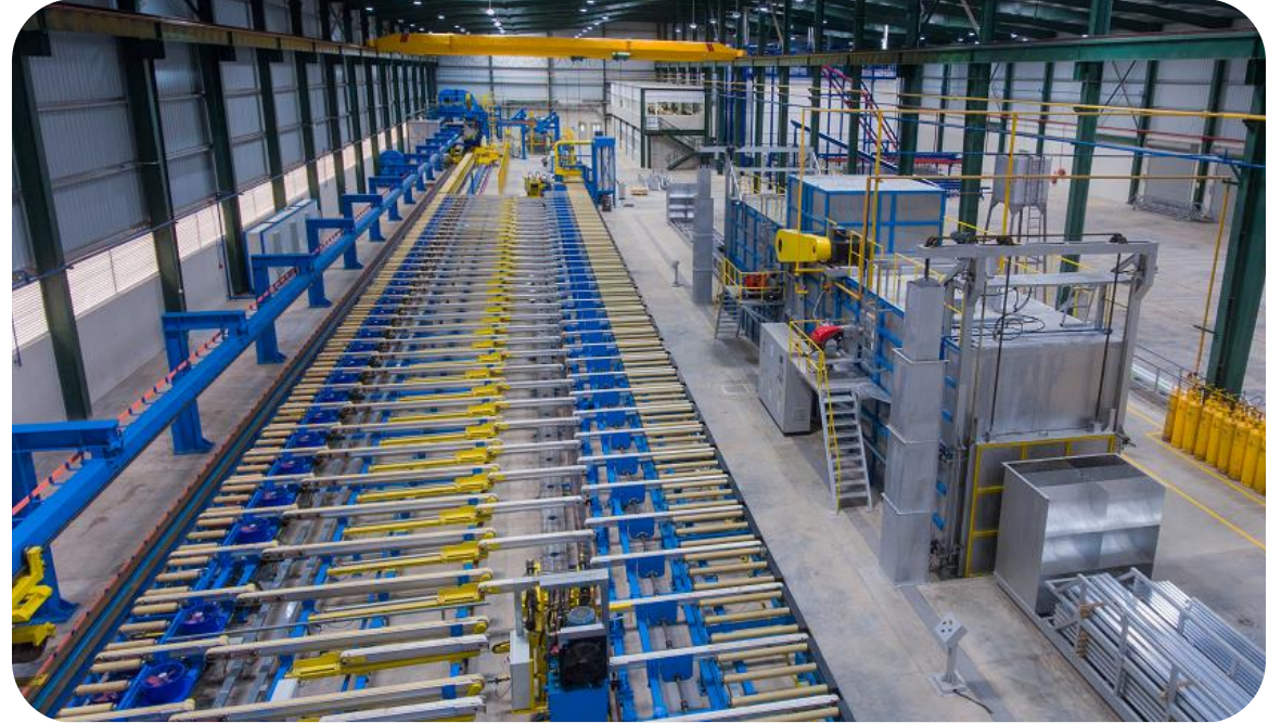
Aluminium Extrusion Plant - Prime Complex Ekala 7" / 8" Ekala (Prezezzi, Italy )Capacity - 12,800 MT p.a
